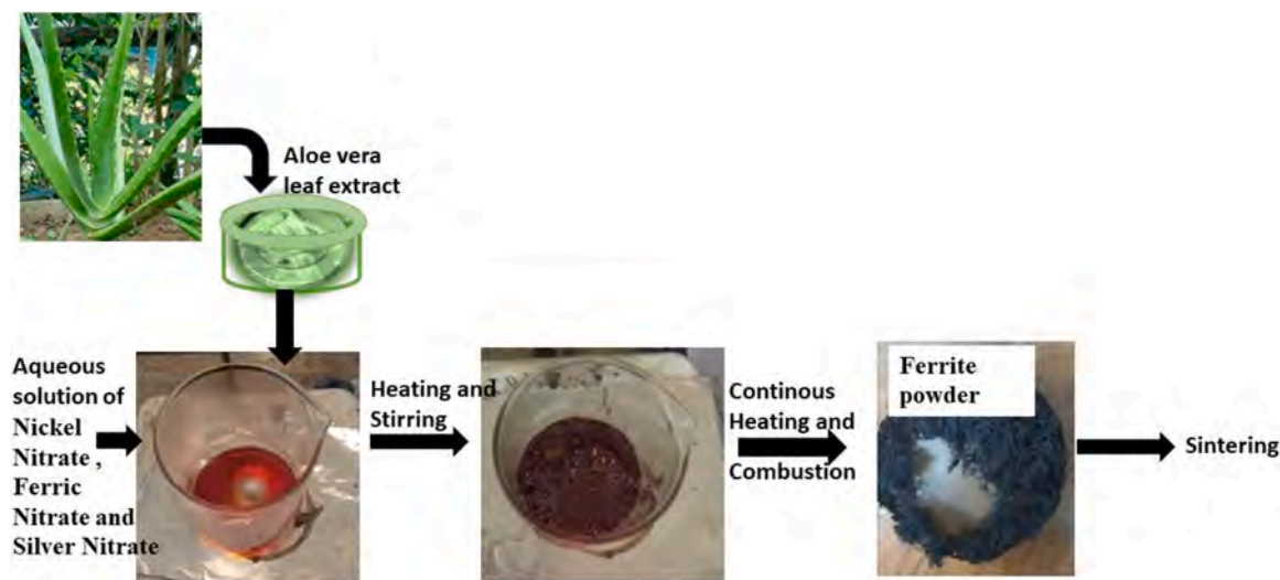
Fig. 1. Flowchart showing the green synthesis assisted sol-gel combustion method.
